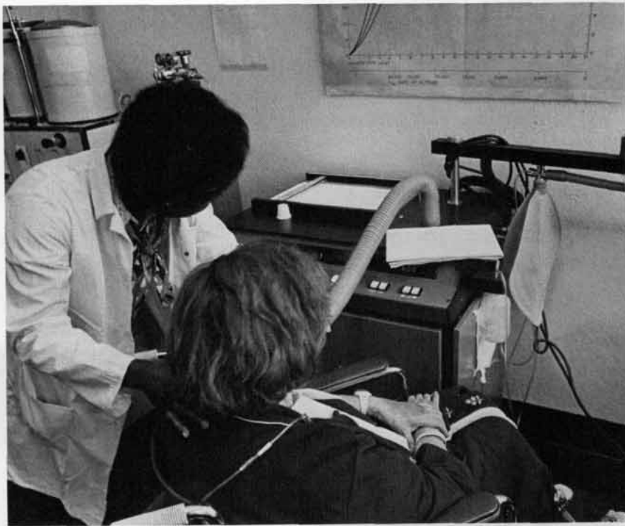
Automated pulmonary function testing allows more tests per hour, simplifies technique and improves quality of data. HP Analyzer shown calculates several measurements in 2 to 3 seconds, prints X-Y plot of washout curve, digitally displays other data on front panel.
