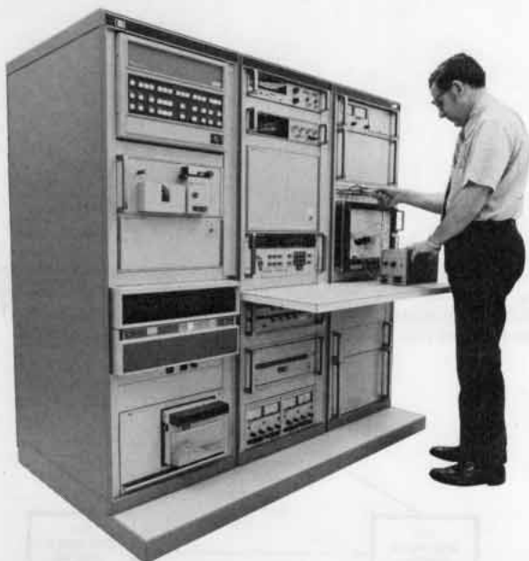
HP9510D Automatic Test System with typical device being readied for testing
