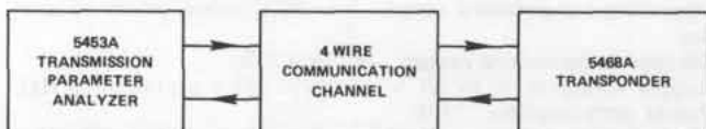
Figure 1. Typical point-to-point measurement. The 5468A is controlled by the 5453A over the channel to be tested.
