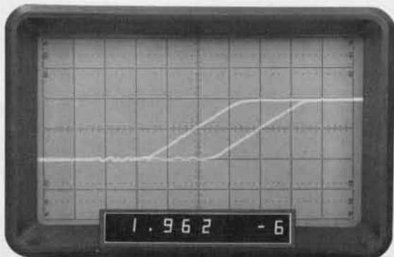
For increased accuracy, the scope is placed in the Delayed Sweep mode to display the two intensified traces alternately. When the two traces are made to coincide using the DEC \rightarrow INC controls, maximum accuracy is achieved ( 1.962 \mu\text{s} , \pm 0.63\% ).
