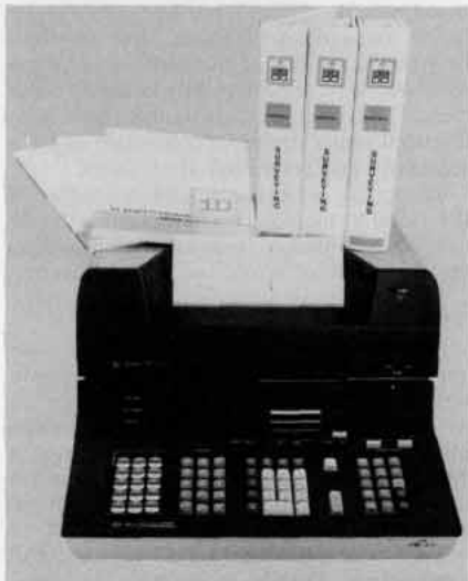
HP9810A Calculator, HP9866A Printer and surveying program library.
